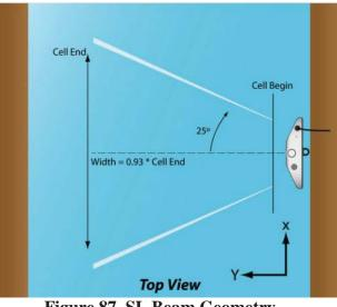
Figure 87. SL Beam Geometry
